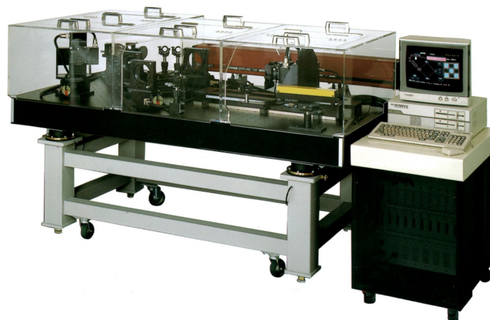
Fig. 6 Externally sealed equipment of exposure system consisted of two-beam interferometer system
